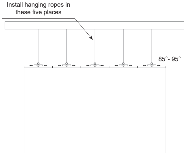
Figure 3.1.1.5 Front side design diagram of hanging installation
