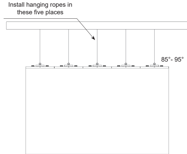
Figure 3.1.1.5 Front side design diagram of hanging installation
