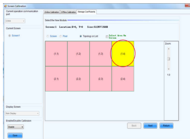
Fig 3-21 Selecting Cabinet for the New Module
